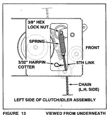
Attach the snow thrower's clutch/idler assembly to the tractor frame by sliding the notched arms at the rear of the assembly onto the two shoulder bolts assembled to the inside of the tractor frame. Lift the front of the assembly so that the sides fit insidethe R.H. and L.H. hanger brackets. Attach the assembly to the brackets using two pivot lock pins and 1/8" hairpin cotters. See figure 14.
